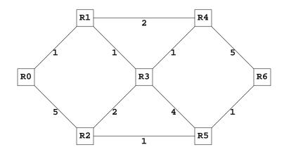
Here is an algorithm for finding the shortest path between two routers. The adjacency table has a zero for every pair of routers that are not connected directly to each other. It also has zero for every router's distance from itself.
